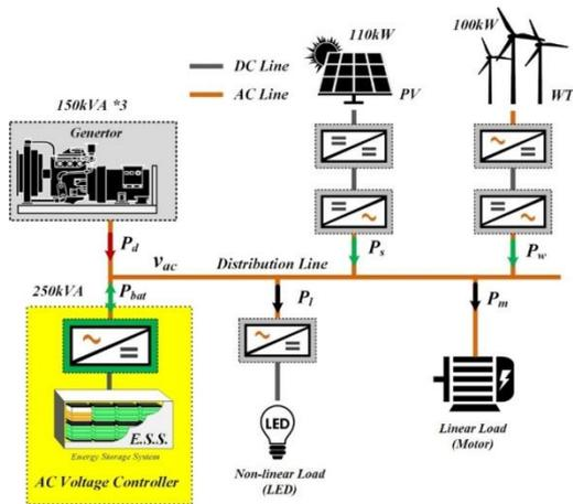
Figure 1: Configuration of Geocha island MG
