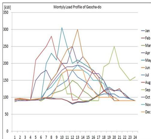
Figure 2: Monthly Load Pattern of Geocha island
