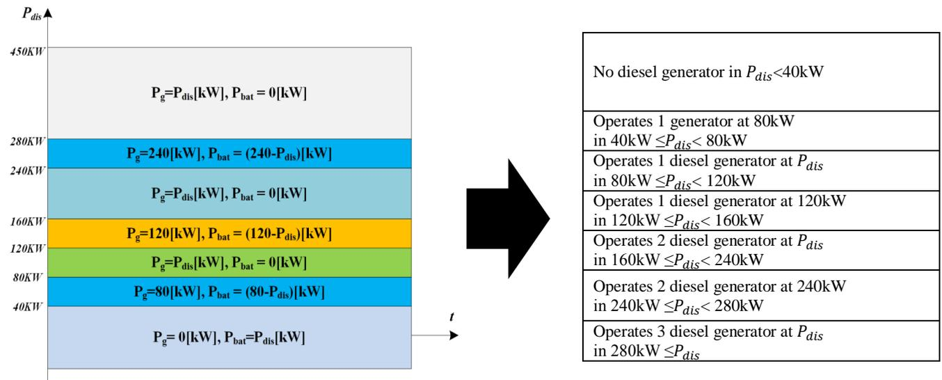
Figure 5: Design of Optimal Operation Algorithm for MG
