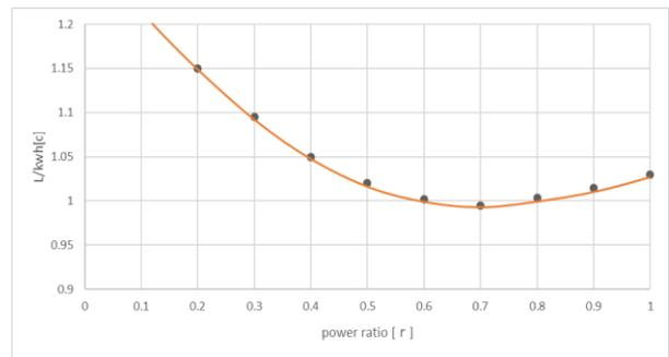
Figure 3: (150kW) Fuel Consumption ratio per Diesel Generator Output Power (curve fitting)
