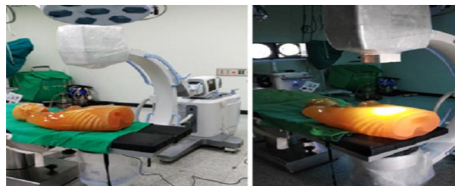
Figure 2: Photograph of C-arm X-ray field display
