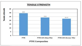
Fig .10:.Tensilse strength of PTFE and PTFE composites
