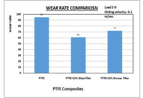
Fig 6:.Wear rate of PTFEand PTFE composites
