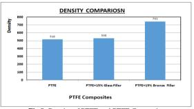
Fig.8:.Density of PTFE and PTFE Composite
