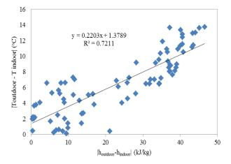
Fig. 5: The correlation between the absolute enthalpy difference and temperature difference of the moist air outdoor and indoor of air-conditioned space
