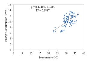
Fig. 3: The correlation between the outdoor temperature and hourly cooling energy consumption
