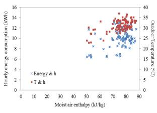
Fig. 4: The relation of outdoor temperature, moist air enthalpy and hourly cooling energy consumption.
