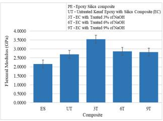
Fig. 7: Flexural modulus of silica modified epoxy composites
