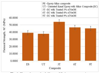
Fig. 6: Flexural strength of silica modified epoxy composites
