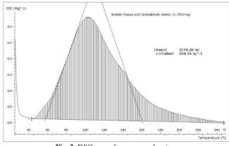
Fig. 3: DSC curve for epoxy and amine
