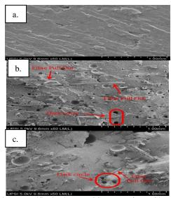
**Fig 8**: Higher magnification images of fracture surfaces of impact specimens (a) Composite ES (silica modified epoxy composite) (b) Composite UT (untreated kenaf silica modified epoxy composite) and (c) Composite 3T (3 % treated kenaf silica modified epoxy composite)
