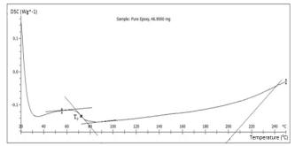
Fig. 4: DSC curve for amine cured epoxy
