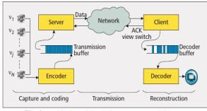
Fig. 3: Multi-view video delivery system architecture
