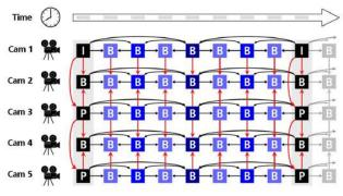
Fig. 2: MVC Prediction Structure with N=5
