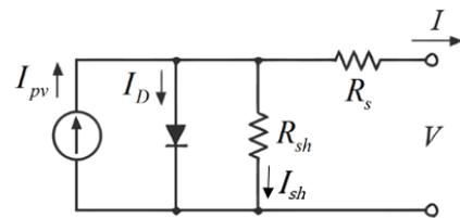
Figure 1: Equivalent Circuit of a Solar cell
