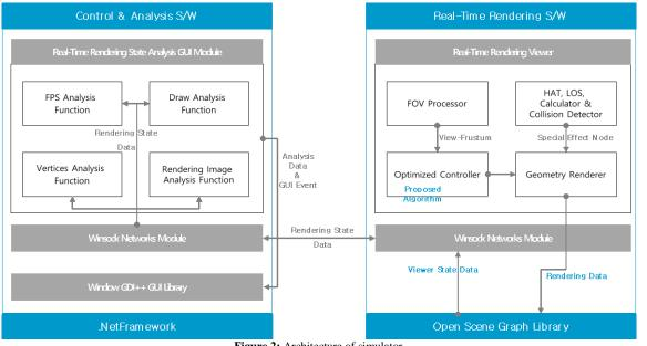
Figure 2: Architecture of simulator
