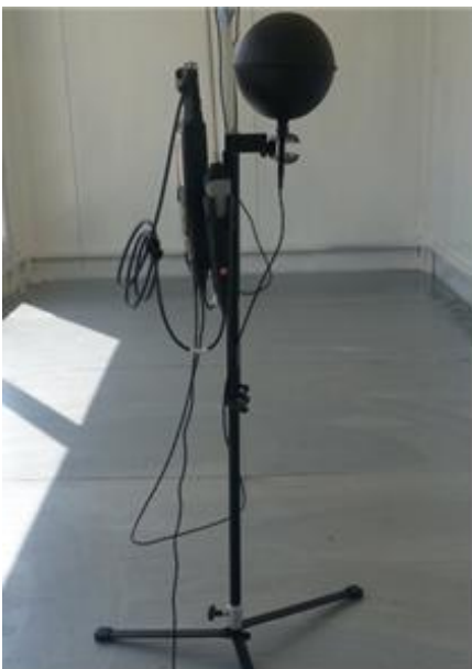
Figure 9: Installation of PMV Measuring Device
