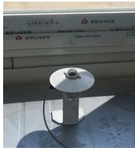
Figure 10: Installation of Pyrheliometer
