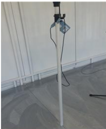
Figure 8: Installation of Thermometer and Hygrometer
