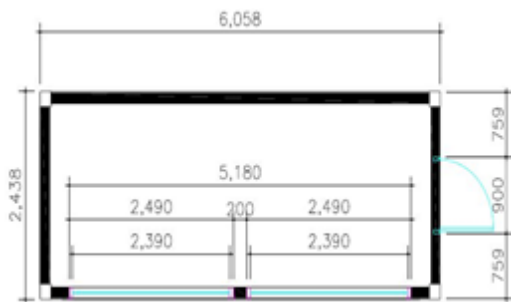
Figure 1: Regular Building (plane view)
