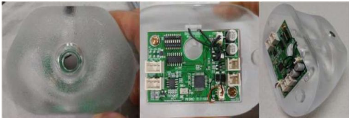
Figure 2: Appearance of a single smart hold, including the control board
