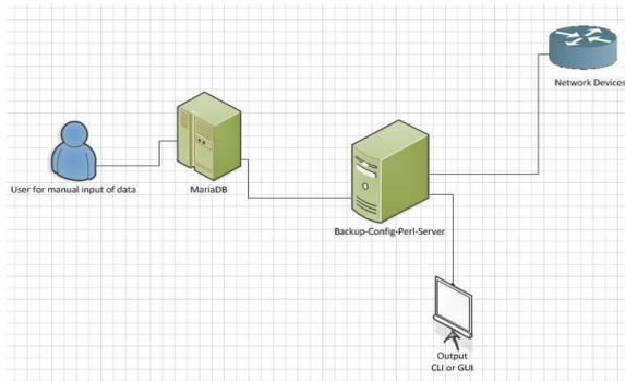
Fig. 1: Logical Diagram of the backup server
