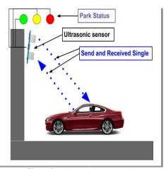
Figure 2:. Ultrasonic Sensor Work
