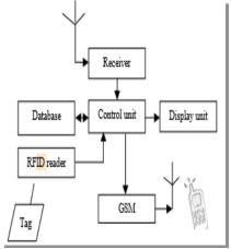
Figure 1:. Block Diagram of Central Control Unit
