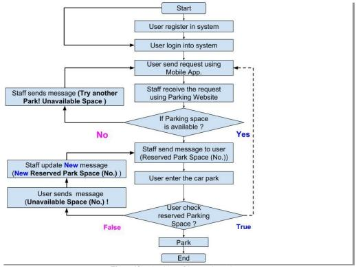
Figure 12:. Algorithm of System Operations.
