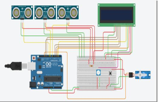
Figure 17: Arduino Electronic Circuit (Smart Parking Manage System)
