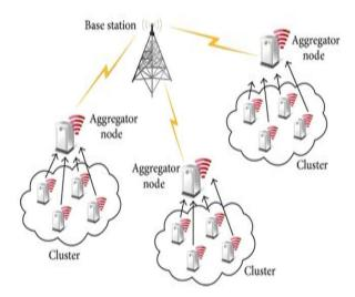
Figure 1:. Data aggregation in WSN
