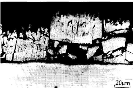
Fig.17: cracks (in the sample (al-5.5%) at the time (600 s)
