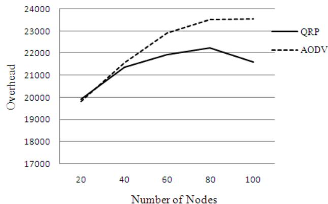
Fig. 8: Routing Overhead
