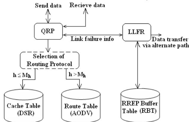
**Fig. 1:** System Architecture. All Letters Used in the Figure Are Explained in the Caption: QRP = Quantum Based Routing Protocol, LLFR = Local Link Failure Recovery, H = Hop Count,  $M_h$  = Minimum Hop Count, DSR = Dynamic Source Routing Protocol, AODV = Ad Hoc on Demand Distance Vector Routing Protocol, RBT = RREP Buffer Table
