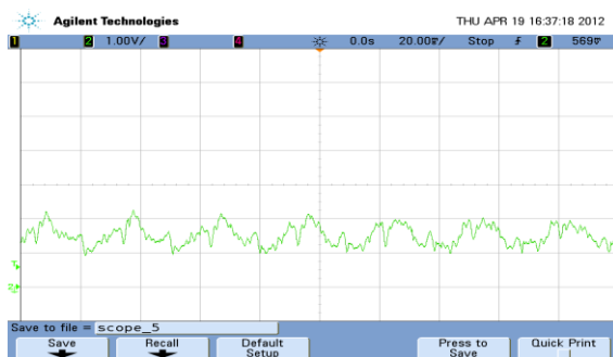
Fig.14: Torque waveform of PI-ILC-SPWM at 100% loading at 2000rpm.
