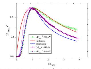
**Fig.5:** Theoretical non-dimensional  $(I/I_{max})^2$  vs.  $t/t_{max}$  plots for instantaneous nucleation from Eq. (1) and progressive nucleation from Eq. (2), to experimental transients current of different potential Fig. 3.
