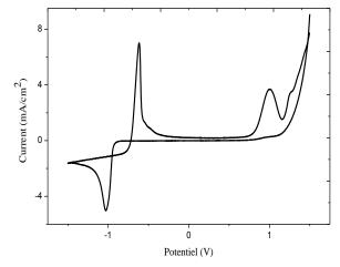
Fig.6: Cyclic voltammogram for Bi electrodeposition on ITO from alkaline electrolyte at potential place (-1.5V to 1.5V/SCE) at scan rate 100mV/s
