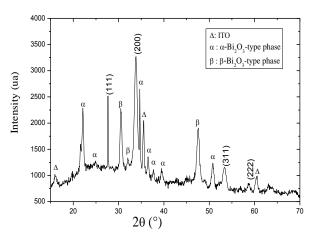
**Fig.8**: X-ray diffraction patterns of  $\delta$ -Bi<sub>2</sub>O<sub>3</sub> thin film.
