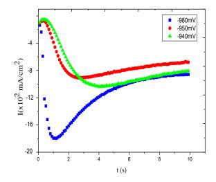
Fig.3: Transients current for Bi electrodeposition on ITO from alkaline electrolyte at different potential
