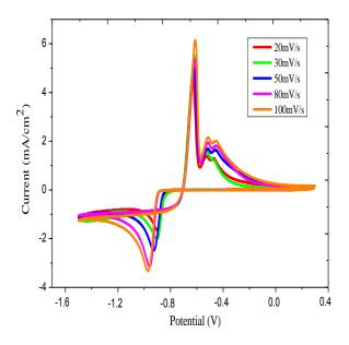
Fig.1: Cyclic voltammograms for Bi electrodeposition on ITO from alkaline electrolyte at different scan rates
