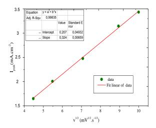
**Fig.2:** The Plot of the cathodic peak current (I <sub>Peak</sub>) versus the square root of the sweep rate  $(v^{1/2})$  for the cyclic voltammograms presented in Fig.1
