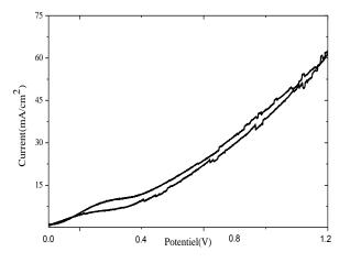
Fig.7: Cyclic voltammogram obtained for a solution 0.25M tartaric acid and 2.5M KOH on ITO at potential place (0 to 1.4V/SCE) at scan rate 100mV/s
