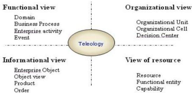
Fig. 1: ISO 19440 views with teleological anchoring.
