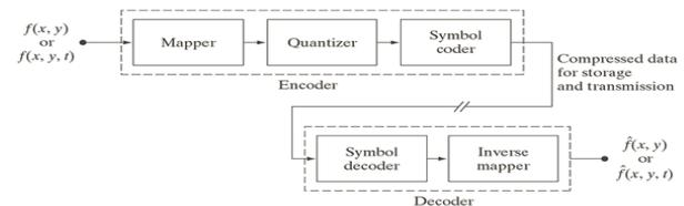
Fig. 2: Functional block diagram of a general image compression system [15].
