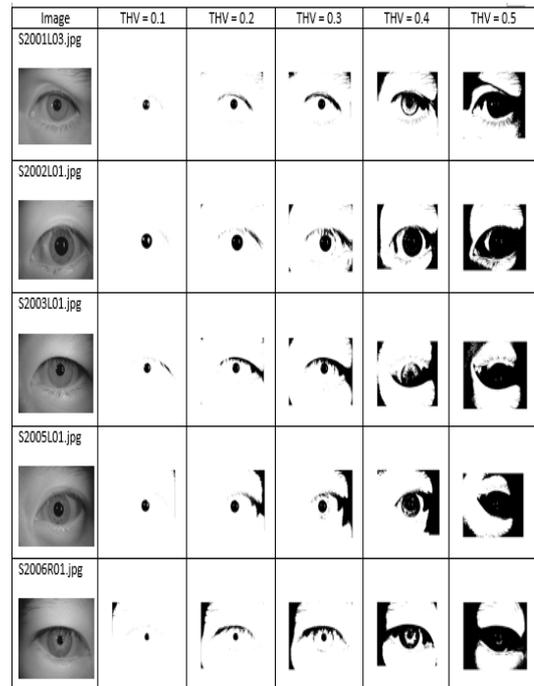
Fig. 12: The result for images in CASIA-Iris-Lamp database
