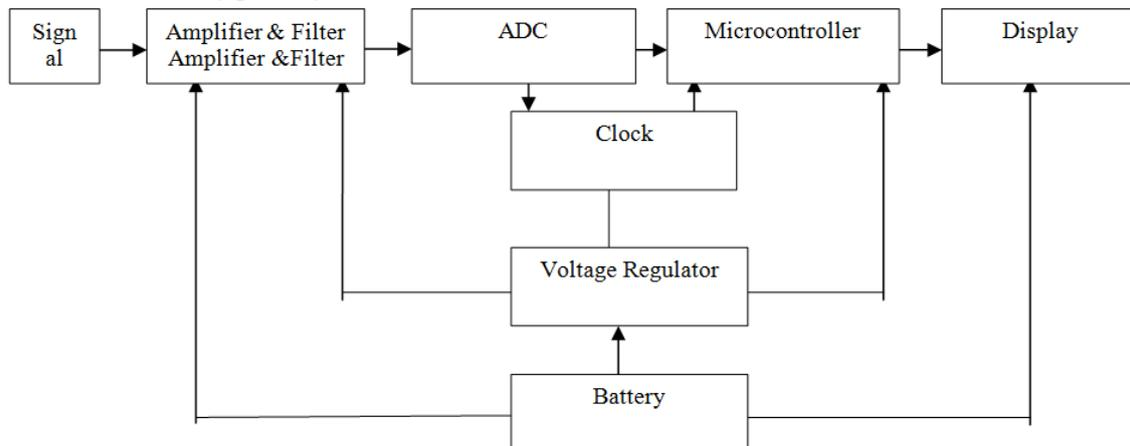
Fig. 3: Heart Rate Monitor System Design. Source: [13].
