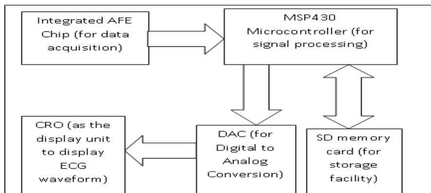
Fig. 2: AFE Chip Based ECG Data Acquisition. Source: [11].
