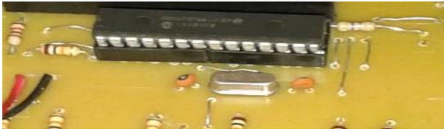
Fig. 9: Signal Processing (Microcontroller)
