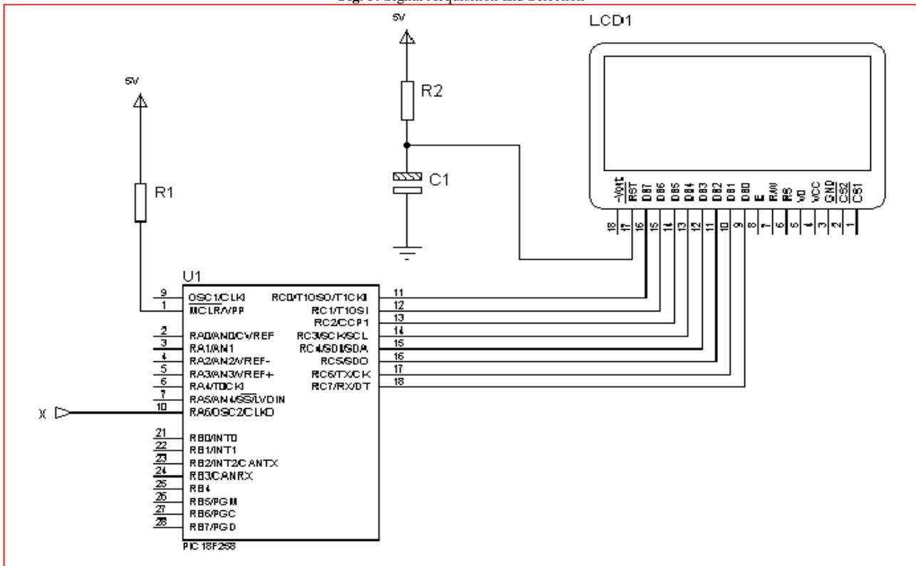
Fig. 6: Signal Processing and Display
