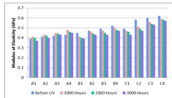
Fig. 4: Modulus of elasticity of WPC samples before and after UV
