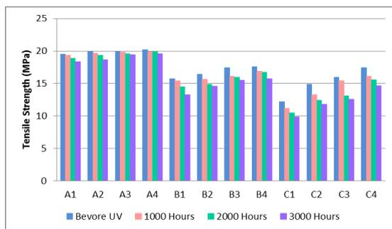
Fig. 3: Tensile strength of WPC samples before and after UV
