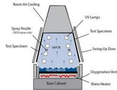
**Fig. 2:** UV accelerated weatherometer
