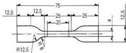
**Fig. 1:** Dimension of dumbbell samples according to ISO 527 (5A): R = radius
