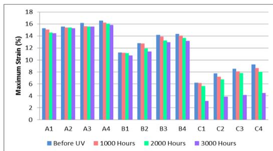
Fig. 5: Maximum strain of WPC samples before and after UV
