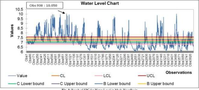
Fig. 4: Result of SPC for Water Level in Muda RiverBasin
