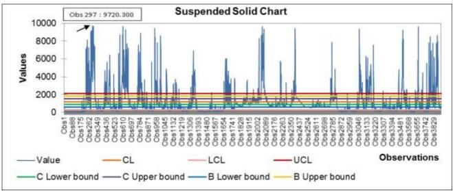
Fig. 3: Result of SPC for Suspended Solid in Muda River Basin
