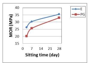
Fig. 4: The values of the fracture coefficient for different ages for both normal epoxy cubes and treatment
