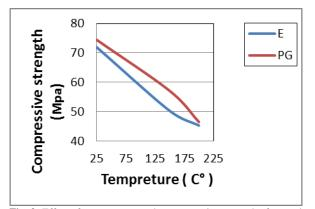
Fig. 3: Effect of temperature on the compressive strength of normal epoxy cubes and treatment
