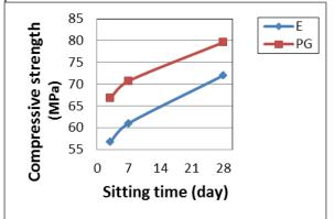
Fig.2: Compression strength of normal epoxy cubes and treatment
