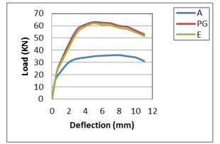
Fig. 7: The load-deflection relationship for ordinary concert beams and Strengthening
