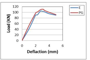
**Fig.5:** The load-deflection relationship after adding the mixture of porcelain and glass to the bonding material.
