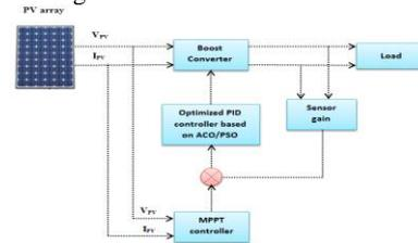
Fig. 2: PV system with proposed MPPT diagram & optimal PID controller.
