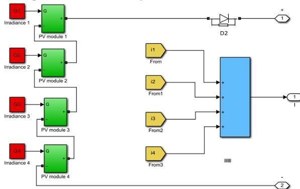
Fig. 4: Block diagram of a PV array with four PV modules.
