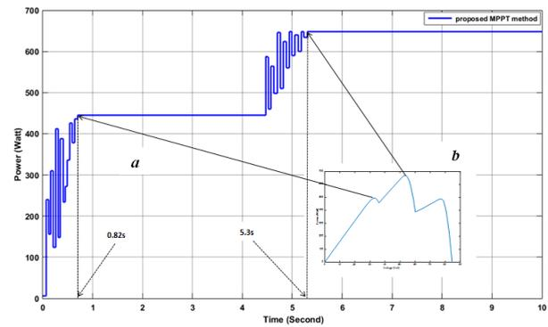
**Fig. 8:** Extracted power using the proposed method (ACO-PSO), under shadow conditions ( $600 \text{ W/m}^2$ ;  $1000 \text{ W/m}^2$ ;  $1000 \text{ W/m}^2$ ;  $800 \text{ W/m}^2$ ).
