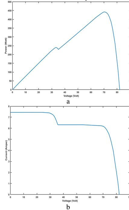
Fig. 4: a) P-V characteristics of the PV array, b) I-V characteristics of the PV array operating under shadow conditions, (400 W/m<sup>2</sup>; 400 W/m<sup>2</sup>; 800 W/m<sup>2</sup>; 800 W/m<sup>2</sup>).
