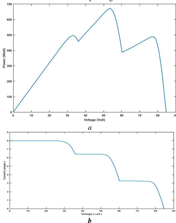
**Fig. 7:** a: P-V characteristics of the PV array, b: I-V characteristics of the PV array, for a system operating under shadow conditions, ( $600 \text{ W/m}^2$ ;  $1000 \text{ W/m}^2$ ;  $1000 \text{ W/m}^2$ ;  $800 \text{ W/m}^2$ ).
