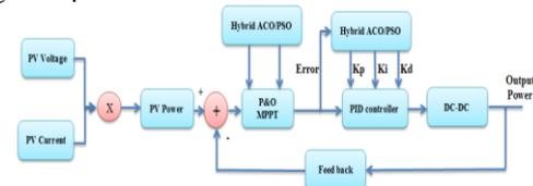
Fig. 1: Block diagram of proposed ACO-PSO based P&O MPPT and PID controller.
