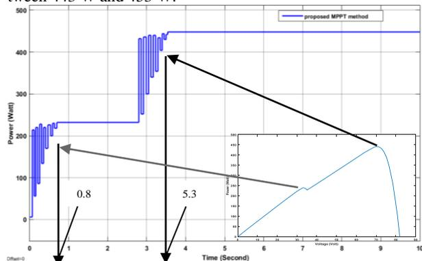
Fig. 5: Extracted power using the proposed method (ACO-PSO), under shadow conditions (400 W/m<sup>2</sup>; 400 W/m<sup>2</sup>; 800 W/m<sup>2</sup>; 800 W/m<sup>2</sup>).
