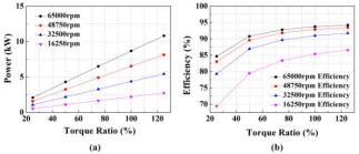
Figure 8: The comparison of the characteristics analysis results of high speed PMSM : (a) Power (b) Efficiency
