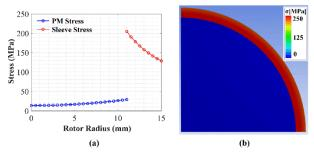
Figure 5: The analytical results of von - mises stress at interference length 13um: (a) PM stress (b) Sleeve stress
