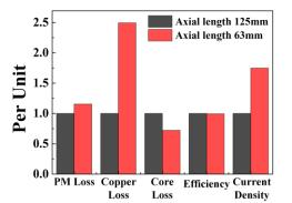
Figure 7: The comparison of the characteristic analysis results according to the D-L ratio
