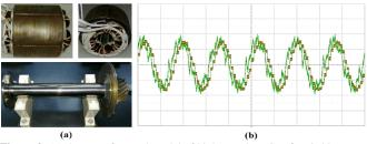
**Figure 9**: (a) the manufactured model of high speed PMSM for air blower, (b) the measurement results of manufactured model
