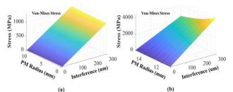
Figure 4: The analytical results of von - mises stress according to interference length and rotor Radius: (a) PM stress (b) Sleeve stress
