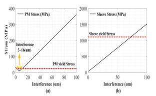
Figure 3: The analytical results of von - mises stress according to interference length: (a) PM stress (b) Sleeve stress
