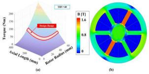
**Figure 2:** The Design Variable Range according to the following Design Specifications: (a) the design variable range (b) design model shape
