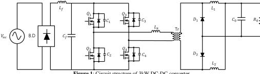
Figure 1: Circuit structure of 3kW DC-DC converter
