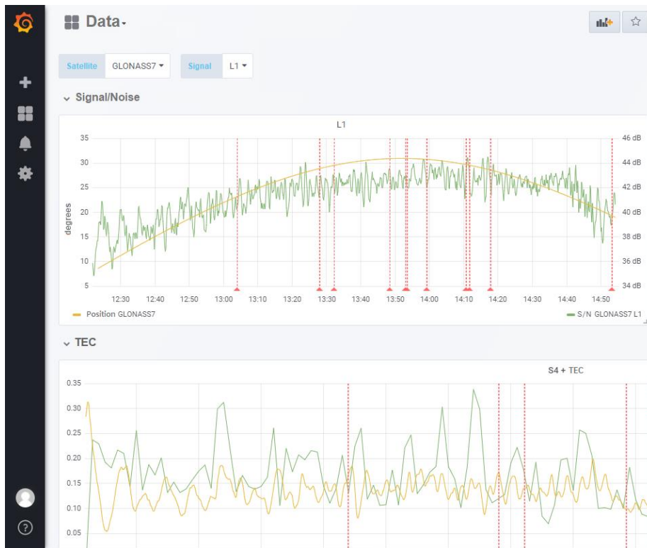
Fig. 7. Ionosphere parameter monitoring based on the evaluation of delays in trans-ionospheric radio wave propagation
