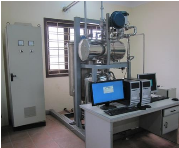
Fig. 2: The Experimental Model of the Level Controller.
