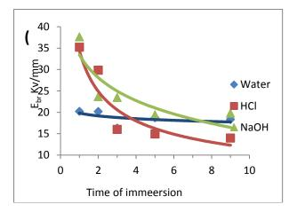
Fig .5: Variation of  $E_{br}$  with time of immersion with different solutions for 1.5 wt (ZrO<sub>2</sub>,Y<sub>2</sub>O<sub>3</sub>) additive ( a.for o.5 kv/s , b.for 5kv/s).
