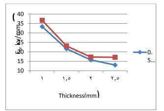
Fig.3: Variation of  $E_{br}$  with thickness for different (ZrO<sub>2-</sub>Y<sub>2</sub>O<sub>3</sub>) additives a.1.5 Wt %, b.4.5 Wt%
