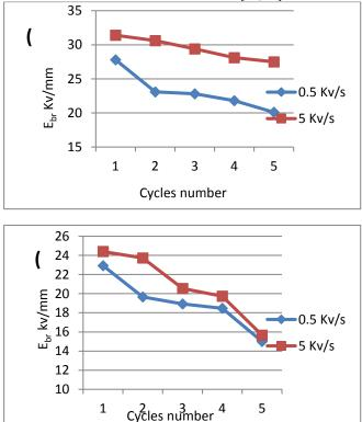
Fig. 4: Variation of  $E_{br}$  with Cycles number without immersion for 1.5 wt% (a.1mm, b.1.5mm) thickness.
