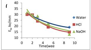
Fig .6: Variation of  $E_{br}$  with time of Immersion with different solutions for 4.5 wt% ( a.for 0.5 kv/s , b. for 5 kv/s)
