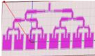
Fig. 5 :Geometry of 8x1microstrip patch antenna array
