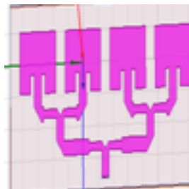
Fig. 4: Geometry of 4x1 microstrip patch antenna array
