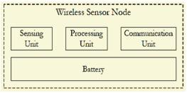
Figure 1: Components of a typical sensor node
