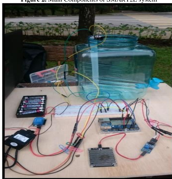
Figure 3. Sensors connected to Arduino Yun
