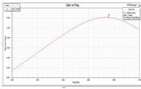
Fig 7: The Gain vs. Frequency Plot
