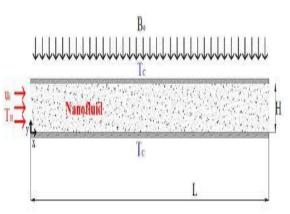
Fig.3 The schematic diagram of computational domain used for simulation of flow in a microchannel with slip velocity.
