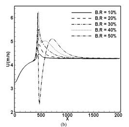
Fig13 Pressure Drop p (a) and velocity  $u_{max}(b)$  for Different Blockage Ratio (B.R) along the channel
