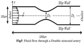
For calculation we considered a Carreau fluid model. Twodimensional Navier-Stokes equations, continuity equation, and momentum equations are applied.
