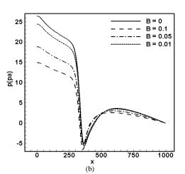
Fig 8: velocity  $u_{max}(a)$  and Pressure Drop p (b) plots for Different Slip velocity co- efficient (B) for n = 0.35 across the channel.
