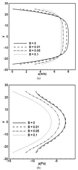
Fig 9: velocity  $u_{max}(a)$  and Pressure Drop p (b) plots for different Slip velocity coefficient(B) for n = 0.35 On throat
