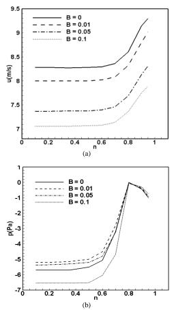
Fig 10: Variation of  $u_{max}$  (a) and Pressure Drop p (b) at different B with respect to n along the channel
