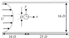
Fig.2: The schematic diagram of computational domain used for simulation of flow past circular cylinder placed inside a channel.
