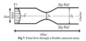
To observe the effect of slip velocity we took different slip length B with respect to n=0.35. In COMSOL a horizontal line is considered to observe the velocity and pressure drop across the channel.
