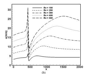
Fig 14: Pressure Drop  $p\left(a\right)$  and  $u_{max}(b)$  plots for Different Re for along the channel
