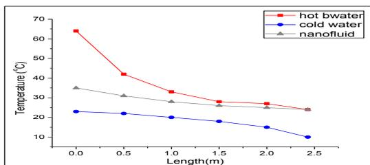
Fig. 4 (b): Temperature variation with length of heat exchanger in counter flow C-H-Narrangement using nano-fluid of 0.1% volume concentration
