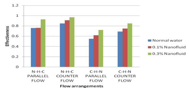
Fig. 7: Effectiveness of the heat exchanger at different flow arrangements
