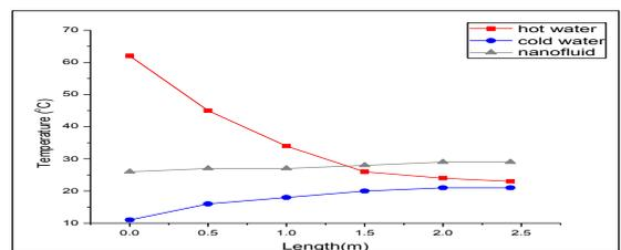
Fig. 5 (b): Temperature variation with length of heat exchanger in parallel flow N-H-C arrangement using nano-fluid of 0.1% volume concentration
