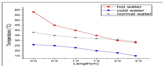
Fig. 4 (a): Temperature variation with length of heat exchanger in counter flow C-H-Narrangement using normal water
