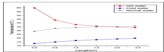
Fig. 3 (a): Temperature variation with length of heat exchanger in parallel flow C-H-N arrangement using normal water
