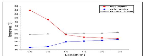
Fig. 5 (a): Temperature variation with length of heat exchanger in parallel flow N-H-C arrangement using normal water
