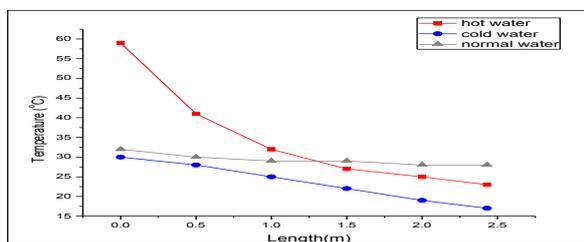
Fig. 6 (a): Temperature variation with length of heat exchanger in counter flow N-H-C arrangement using normal water
