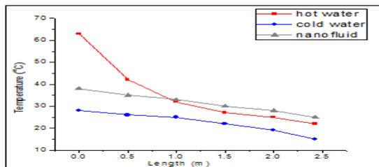
Fig. 4 (c): Temperature variation with length of heat exchanger in counter flow C-H-N arrangement using nano-fluid of 0.3% volume concentration
