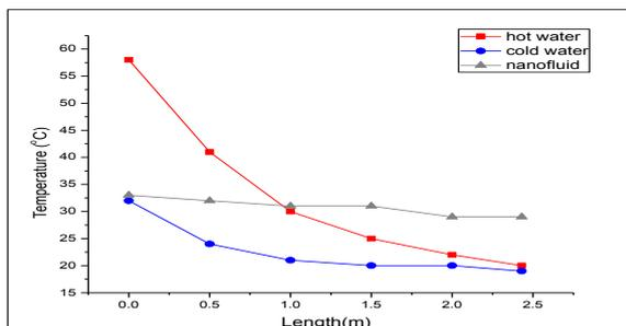
Fig. 6 (c): Temperature variation with length of heat exchanger in counter flow N-H-C arrangement using nano-fluid of 0.3% volume concentration
