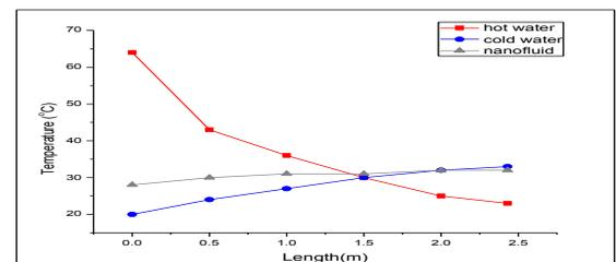
Fig. 5 (c): Temperature variation with length of heat exchanger in parallel flow N-H-C arrangement using nano-fluid of 0.3% volume concentration
