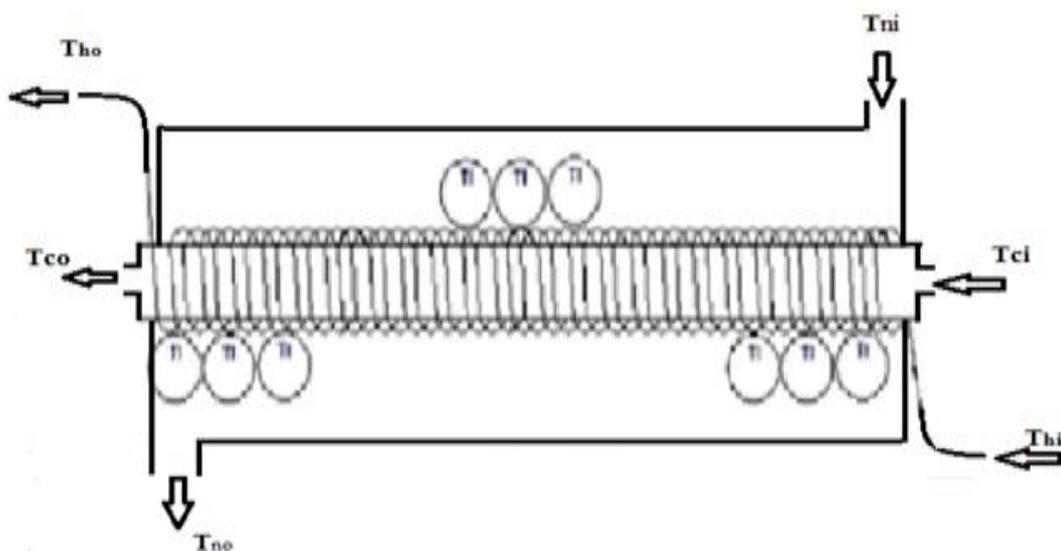
Fig.1 (b): Schematic diagram for TCH pipe heat exchanger with C-H-Nparallel flow
