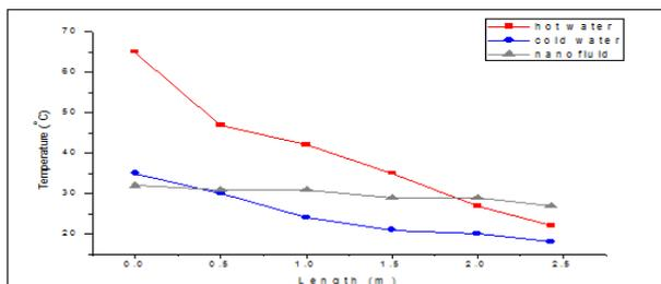
Fig. 6 (b): Temperature variation with length of heat exchanger in counter flow N-H-C arrangement using nano-fluid of 0.1% volume concentration
