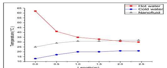
Fig. 3 (b): Temperature variation with length of heat exchanger in parallel flow C-H-N arrangement using nano-fluid of 0.1% volume concentration
