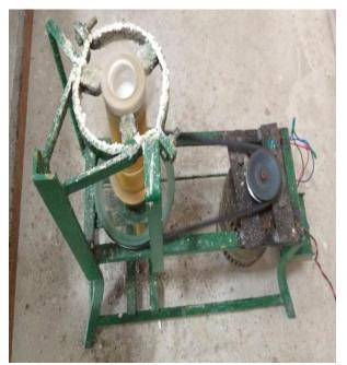
Fig.2: Rotation of mould at 250 rpm
