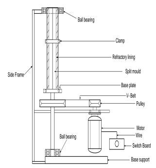
Fig.1: Schematic diagram of experimental setup
