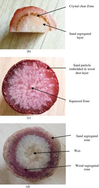
Fig.3: Centrifugal casting of prototype model at 250 rpm (a,b) 0.5 vol% wood and 0.02 vol% of sand, (c) 0.10 vol% of wood and 0.02 vol % of sand, (d) 0.16 vol% of wood and 0.19 vol% of sand
