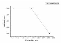
Fig 8: Flux weight vs bead width of SiO<sub>2</sub>
