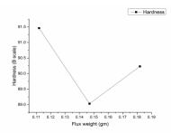
Fig14: Flux weight vs Hardness of CdCl2
