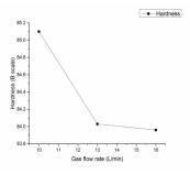
Fig15: Flowrate vs Hardness of without flux
