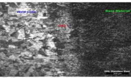
Fig17: Microstructure of base material, weld zone and HAZ
