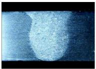
Fig 1: Specimen 16, Weld penetration-5.08mm, Bead width-6.08mm, D/W ratio-0.83
