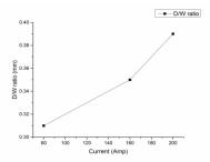
Fig 10: Welding current vs D/W ratio of without flux
