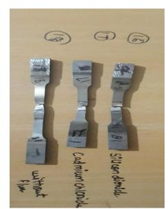
**Fig 16:** Tensile photograph of 304L stainless steel (16) with use of oxide flux(17) with use of chloride flux(18) with the use of flouride flux
