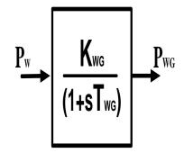
Fig.3: Transfer function model of wind generator system
