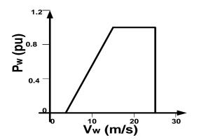
Fig.2: Curve forpower generated by wind turbine versus speed of wind
