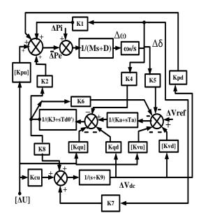
Fig.4: Modified Heffron-Phillips model including UPFC
