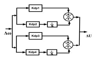
Fig.5: The dual PI controller
