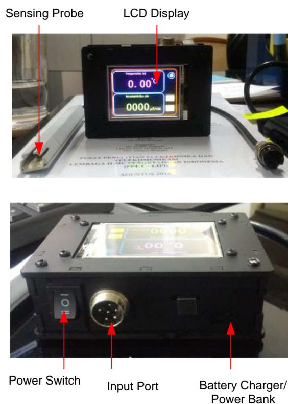
Fig. 4: The developed portable instrument consisting of a sensing probe and a data logger
