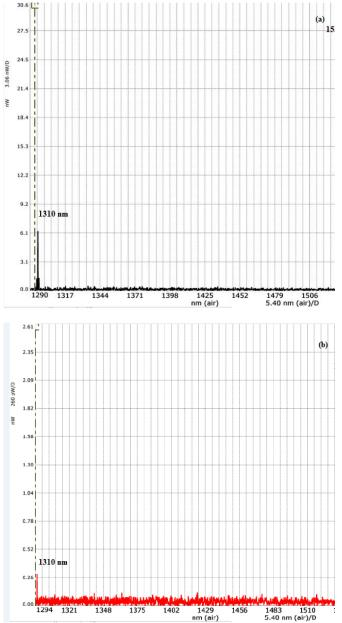
Fig. 6: The All Link Dispersion Effect of Length 3 Km (a) Without Using FBG, (b) With Using FBG.
