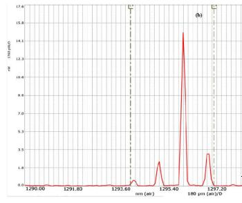
Fig. 5: The 1310 nm Link Dispersion Effect of Length 3 Km (a) Without Using FBG, (b) With Using FBG.
