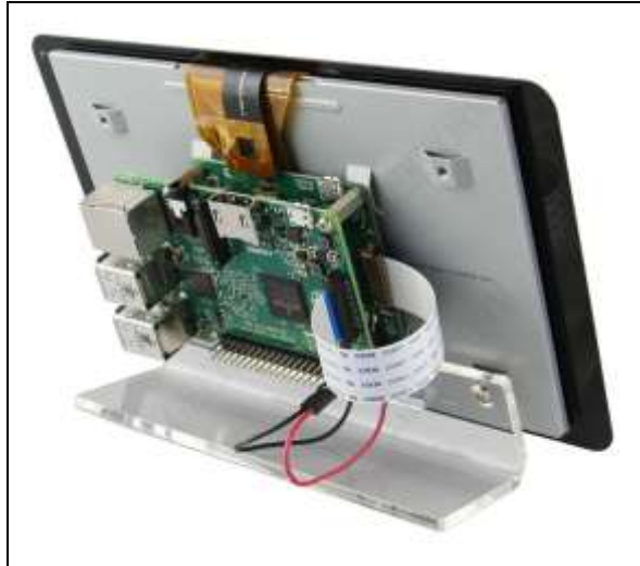
Fig. 7: Integration of Raspberry Pi and 7-Inch Touch Screen
