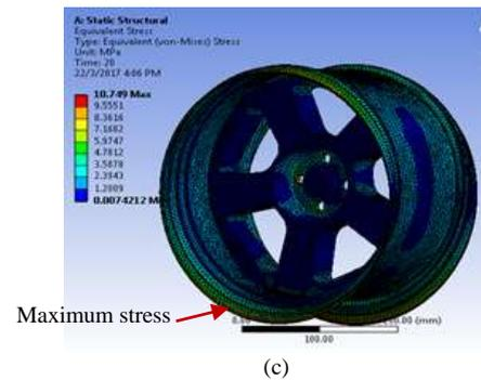
Fig. 6: Stress distribution on (a) aluminium alloy, (b) magnesium alloy and (c) titanium alloy wheels
