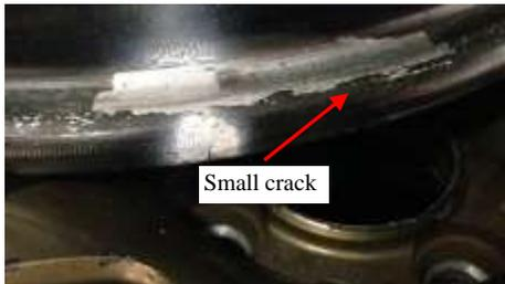
**Fig. 1:** Alloy wheel of a 1200 cc national automobile with a small crack on the outer surface of the rim
