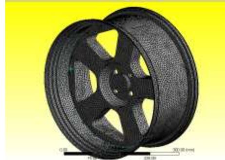
**Fig. 3:** Finite element model with mesh
