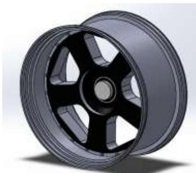
**Fig. 2:** Isometric view of a 3D model design of an automobile alloy wheel
