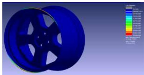
Fig. 7: Number of cycles to failure for aluminium alloy wheel
