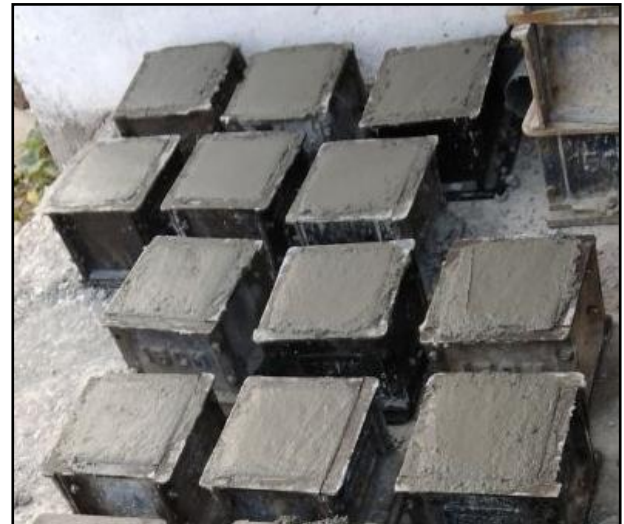
Fig. 1: Casting of Cubes after Obtaining Uniform Mix in Pan Mixer.
