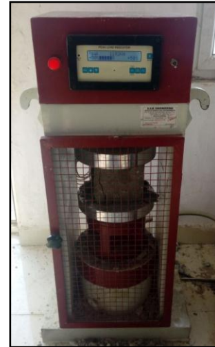
Fig. 2: Testing of Cube as Per IS 516.
