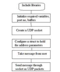
Fig. 7: Flowchart for socket programming (Linux)
