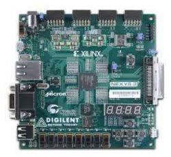
Fig. 2: Xilinx Nexys 3 FPGA board
