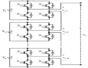
Fig.1: circuit diagram of multilevel inverter
