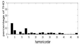
Fig.6: Harmonic order with its distortion with modulation index 0.66
