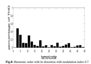
From fig (7) 3rd harmonic voltage is 4.2V and 5th order harmonic voltage is 5.8V.From fig (8) 3rd o harmonic distortion is 0.48 and 5th harmonic distortion is 0.3 with modulation index 0.7.In this case the overall THD is found out 6.6%.As compare with modulation index 0.66, in this case 5th order harmonic peak voltage and percentage of THD is more.
