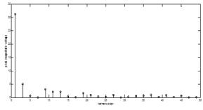
Fig.5: Peak magnitude voltage VS harmonic order with modulation index  $0.66\,$
