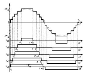
Fig.2: Output voltage waveform of an 11 level inverter, with unequal DC sources
