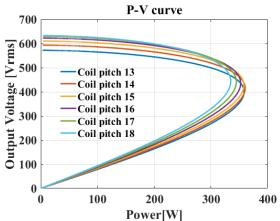
Figure 6: Power-voltage curve according to coil pitch
