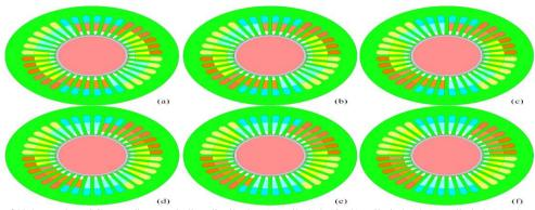
Figure 2: Structure of high-speed PMSG according to winding distribution:(a) coil pitch 13, (b) coil pitch 14, (c) coil pitch 15, (d) coil pitch 16, (e) coil pitch 17, (f) coil pitch 18
