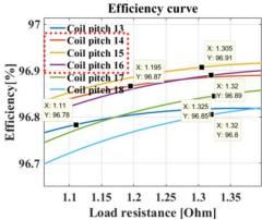
Figure 11: Efficiency according to coil pitch
