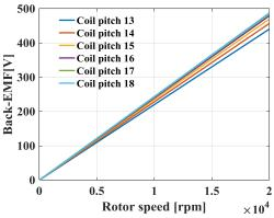
Figure 5: Back-EMF according to rotor speed
