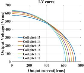
Figure 7: Current-voltage curve according to coil pitch
