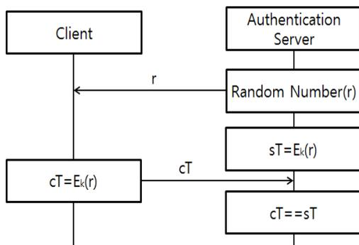
Figure 2: Challenges-Response Based Authentication Model
