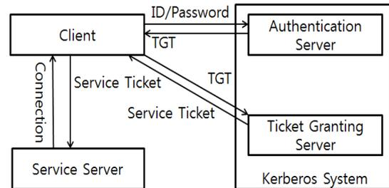
Figure 3: Kerberos System Based Application Model
