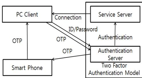
Figure 5: Smart Phone Based Authentication
