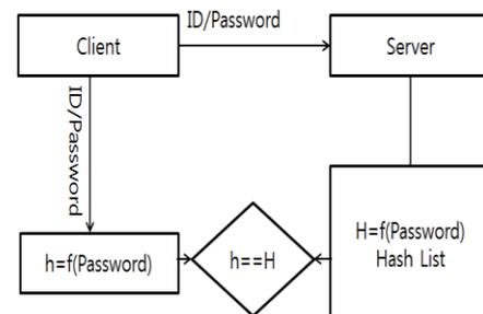
Figure 4: Password based Authentication Model Using One-Way Function
