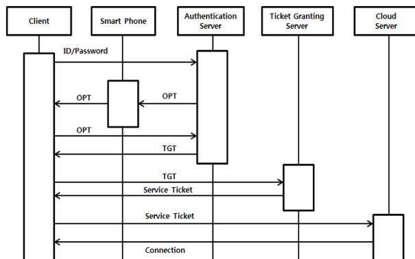
Figure 6: Kerberos System Based Security Model Using Two Factor Authentications for Cloud Computing
