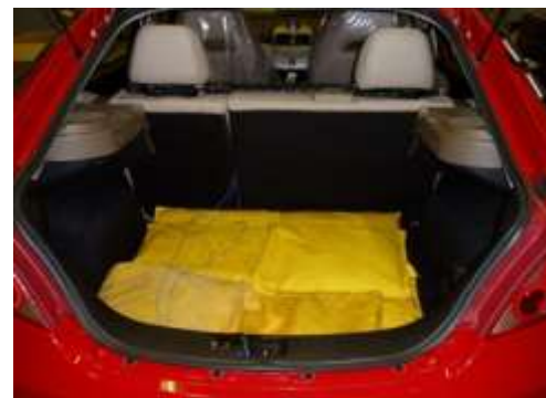
Fig. 4: The sandbag (yellow colored) represents the load weight on the rear of the vehicle Source: National Automobile Company Bhd.
