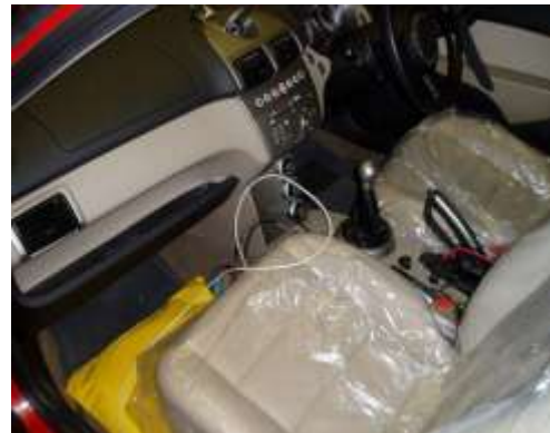
Fig. 3: The sandbag (yellow) represents the weight of the passenger Source: National Automobile Company Bhd.
