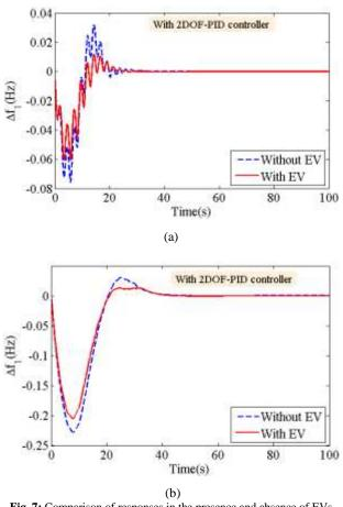
Fig. 7: Comparison of responses in the presence and absence of EVs (a)  $\Delta f_1$  vs time with simultaneous perturbation in two areas (b)  $\Delta f_1$  vs. time with simultaneous perturbation in all the areas
