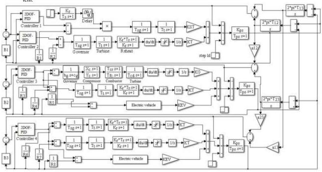
Fig. 1: Transfer function model of unequal three area multi-source system embedded with electric vehicle
