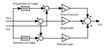
Fig. 3: Schematic diagram of 2DOF-PID Controller
