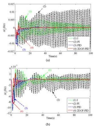
Fig. 4: Comparison of responses of 2DOF-PID, PID, PI, and I controllers (a)  $\Delta f_2$  vs time
