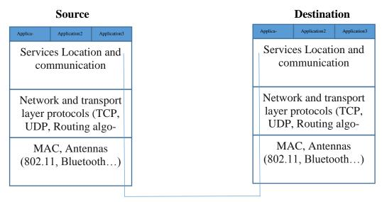
Fig. 1.3: Architecture of wireless adhoc network [1]
