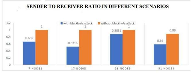
Fig. 6.2: Sender to receiver ratio comparison in different scenarios
